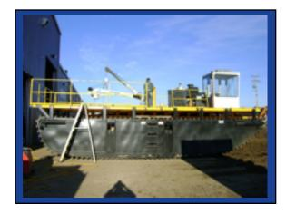
STEERING: STANDARD TRAVEL CONTROLS ONE FOR EACH TRACK IS USED. CAPABLE OF COUNTER ROTATING BY PUSHING ONE LEAVER AND PULLING THE OTHER WITHOUT MOVING BACK AND FORTH OR USING ANOTHER PIECE OF EQUIPMENT FOR ASSISTANCE
